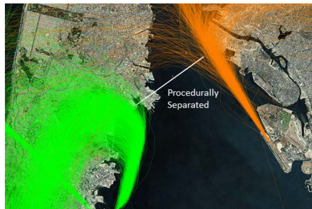
Figure 8 – OAKLAND SID (Orange) and SSTIK SID (Green). As published, the two procedures are procedurally separated.
