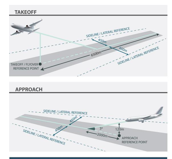
Measurement locations can vary with aircraft stage, number of engines, and lift mechanism. Some types are certificated based on level flyover.
